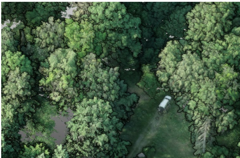
Colorized 3D point cloud derived from UAV-LiDAR data.
